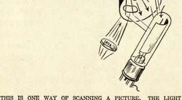
THIS IS ONE WAY OF SCANNING A PICTURE. THE LIGHT REFLECTED FROM EACH SPOT OF THE PICTURE SHINES UPON THE PHOTO-ELECTRIC CELL ON THE RIGHT.
