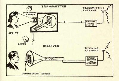
scope, the tube has an electron gun down in its narrow neck. The top of the tube is flat. It is made of a material that acts just the opposite from photo-electric material. Instead of producing electricity when light falls upon it, this material 33 gives out light when electricity strikes it. In other words, it is luminescent. This luminescent material forms the screen on which the moving pictures are produced.
