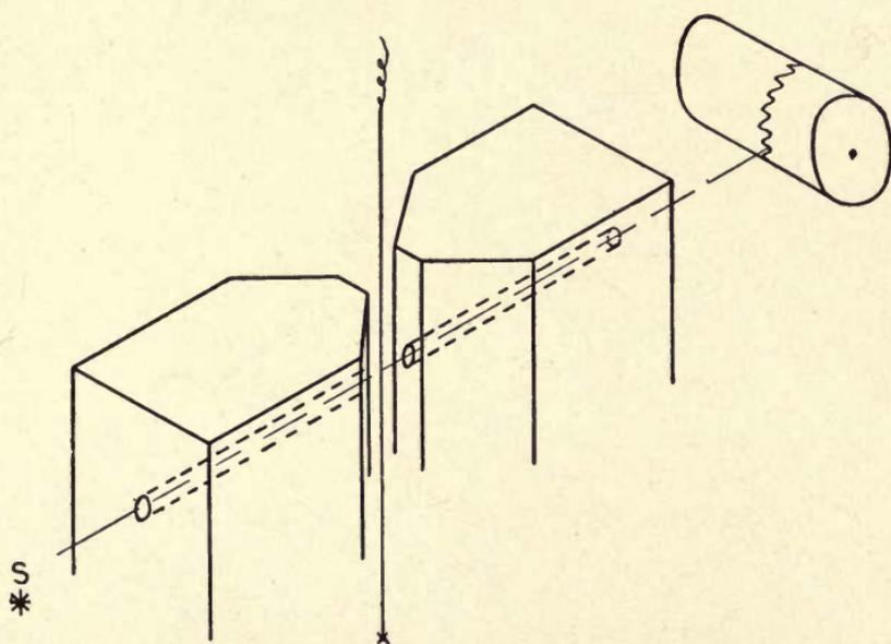
FIG. 41.—The arrangement of parts of a string oscillograph is shown above.
