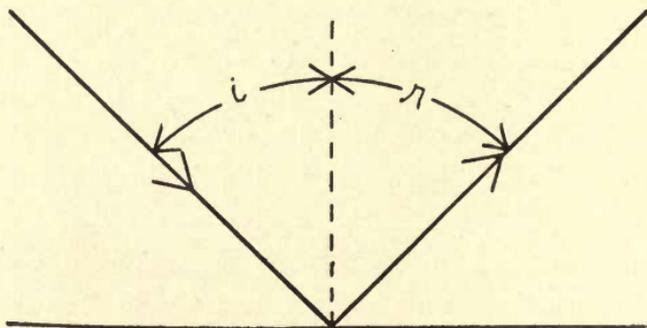
FIG. 9.—For a mirror the angle of incidence ( $i$ ) of a light beam is equal to the angle of reflection ( $r$ ).
