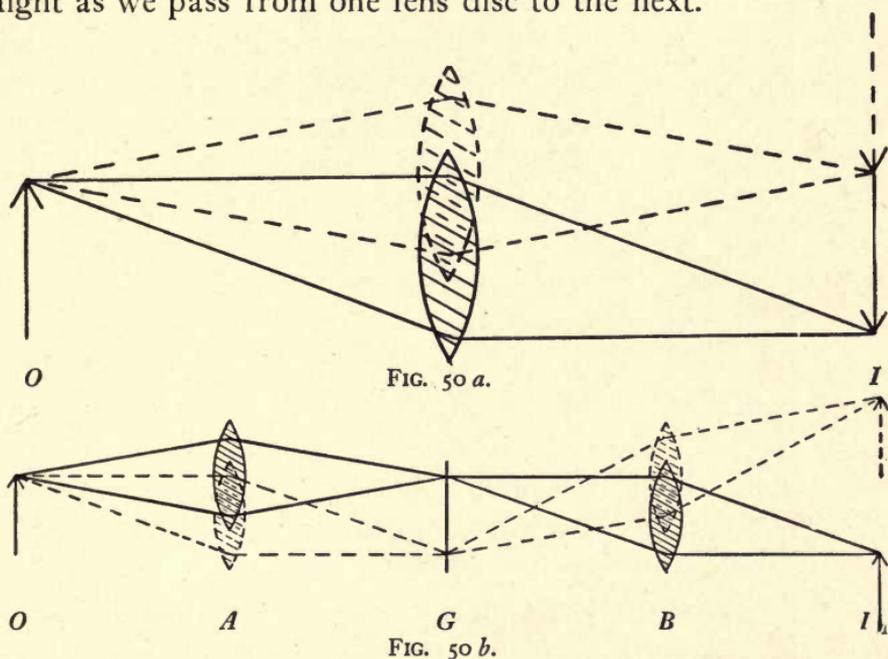
FIG. 50.—Moving a single lens will displace the image *I* as shown in *a*, but moving two lenses *A* and *B* in opposite directions will give a greater displacement as shown. *B* picks up the image from the ground glass screen *G*.
