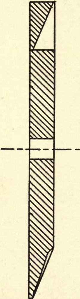
FIG. 51 a.—A cross-section of the Jenkins scanning disc.
