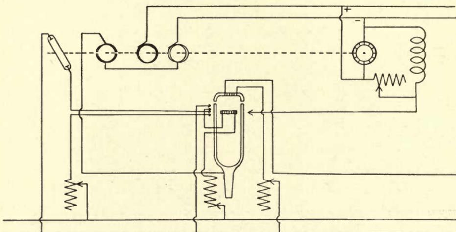
FIG. 53.—Schematic diagram of circuit used for synchronization in the Ranger system. Neon tube, at upper left, is connected to motor shaft, at upper right, and is used as a stroboscope.
