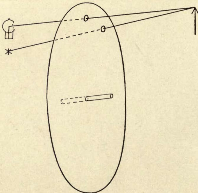
FIG. 84.—A Baird system whereby a spot of light is projected to the exact spot of the scene at the moment being scanned, by a double use of the scanning-disc.
