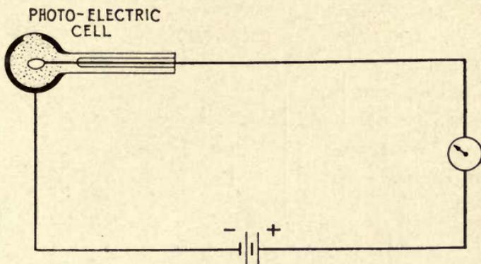
FIG. 32a.—The essentials of a photoelectric cell circuit.
