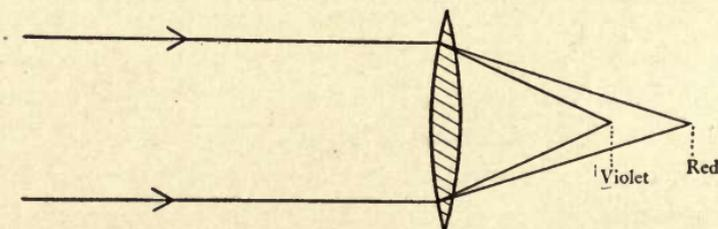
FIG. 16.—Different colors will focus different distances from the lens unless it has been specially corrected for this fault by being made up of different kinds of glass cemented together.
