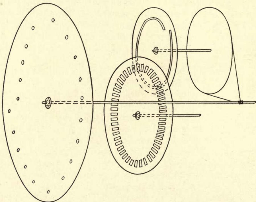
FIG. 47.—Scanning arrangement used in the Baird system.
