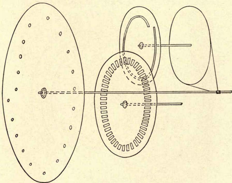
FIG. 76.—Scanning arrangement used in the Baird system.
