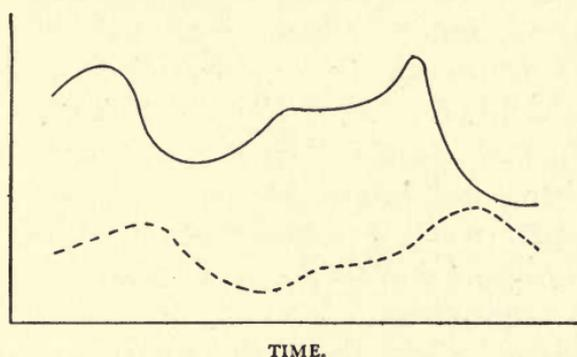
FIG. 25.—Comparison of the fluctuation of light intensity (solid line) and conductivity of a typical selenium cell (dotted line). Note time lag and rounding of conductivity curve.
