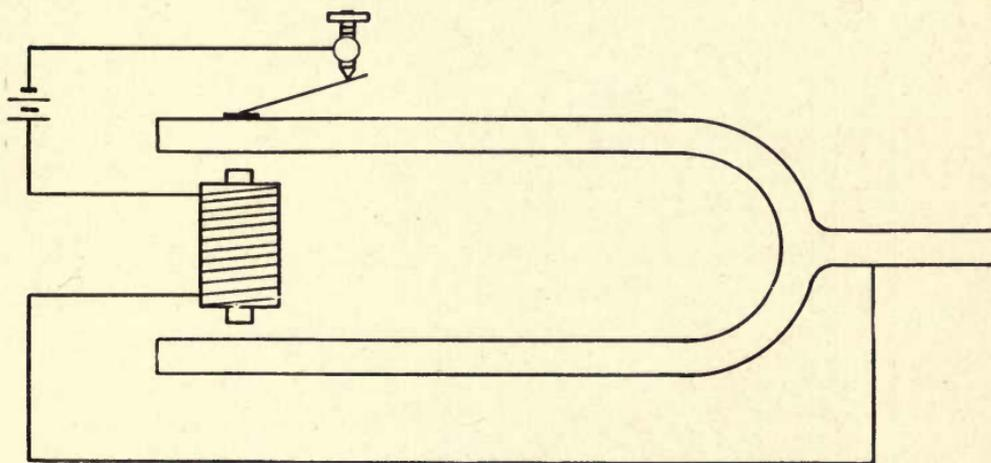
FIG. 52.—Electrically driven tuning fork.
