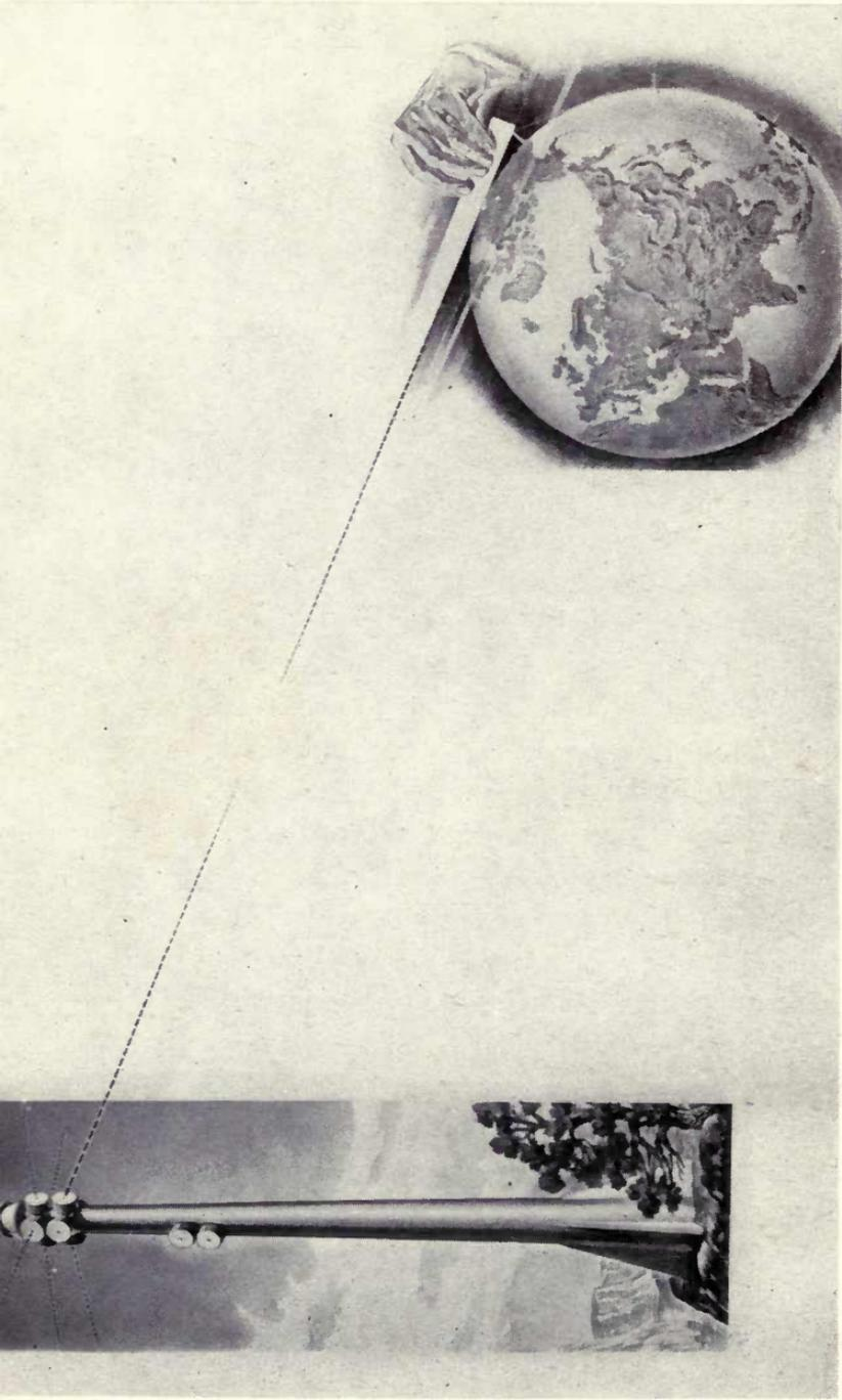
Microwaves, which carry the television pictures and sound, travel on a straight line and therefore touch the earth over a limited radius of approximately 30 to 50 miles. That is why radio relay stations are used to intercept the waves and "bend" them around the curvature of the earth; and why high receiving antennas are sometimes needed to reach up to capture the overhead waves.
