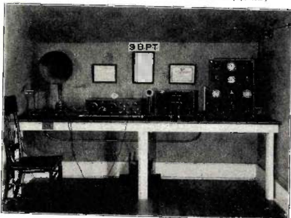
Station 9BPT, owned and operated by Harry D. Clingenpeel, Flora, Ind. The transmitter is a 100-watt C.W. and a 10-watt phone set. The Hartley circuit is used and the (300 prior to Ray-don 1,000-volt A.C. motor generator. Plate current is 250 milliamperes. The receiving circuit consists of a Grebe CR-3 and a 1BGF short wave low loss tuner. The aerial is a wire cage 22 feet long and 30 feet and 25 feet high with lead-in or low end. The counterpoise is fan type, and extends radially beneath the cage for 20 feet.
