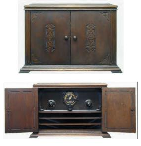
made by or expressively for Magnavox audios, capacitors, tube sockets and variometers. Its one-dial tuning is almost unique for 1924.
