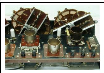
Variometer detail...note the white, porcelain knobs for the "variable ratio condensers"
