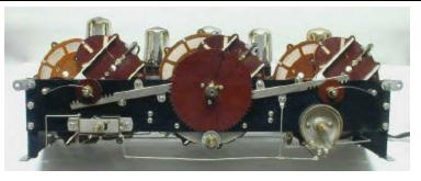
"Single dial" tuning mechanism detail
