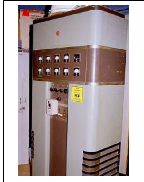
Left: The BTA-250L was used as the backup transmitter for WMID-AM 1340 (Atlantic City) - automatically came on if main transmitter failed.
