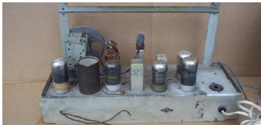
"There was an empty octal socket which I thought was from a missing tube."
