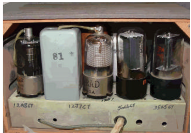
A "neat" way to eliminate the 409's original resistance line cord. The original tube lineup of 6A8GT, 6J7GT, 25L6GT and 25Z6GT has been changed to a 12A8GT, 12J7GT, 50L6GT and 35Z5GT with only one tube socket modification required. The museum's 409 "Sparton" tube lineup will remain "original."
