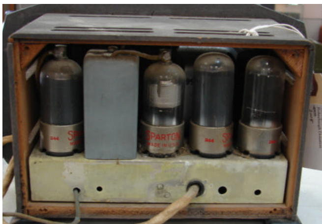
A "neat" way to eliminate the 409's original resistance line cord. The original tube lineup of 6A8GT, 6J7GT, 25L6GT and 25Z6GT has been changed to a 12A8GT, 12J7GT, 50L6GT and 35Z5GT with only one tube socket modification required. The museum's 409 "Sparton" tube lineup will remain "original."
