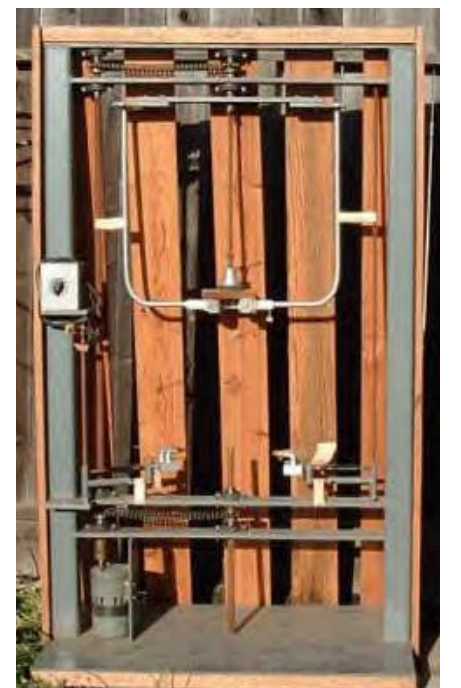
The vertical lathe, used to rotate the CRT shell as the new neck and stem are attached.
