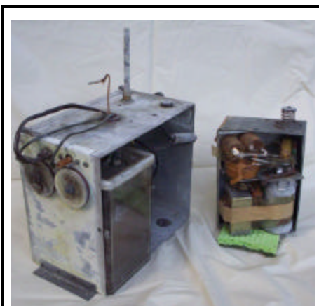
Close-up of the battery case with the vibrator circuitry exposed. The battery is dried out so I'll leave it that way for safety. There's an asbestos backing on the side support which deserves caution. The copper oxide rectifiers may be seen on the upper left side of the battery case. Note the spring shock mount for the vibrator case.
