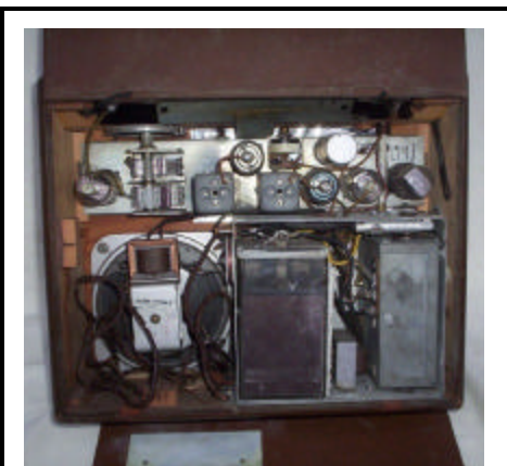
Rear view of the GE LB530. Note the battery and vibrator case in the lower right.
