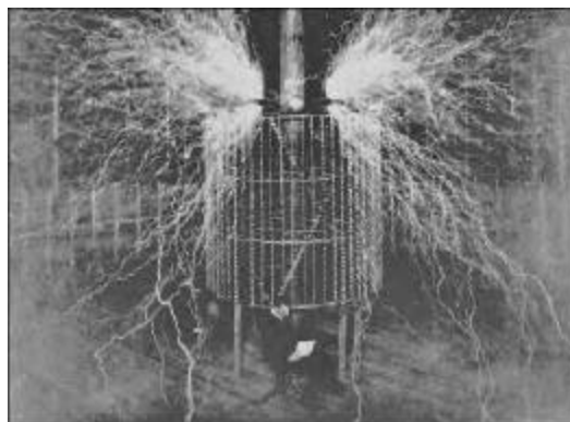
Nikola Tesla in a popular multiple exposure photo in 1899, as a Tesla coil discharged millions of volts. He is seated inside a circular framework 51 feet in diameter, which supported the primary and secondary conductors of the largest Tesla coil ever built, at his Colorado Springs experimental station.
