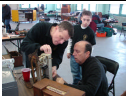
Walt Heskes located a bad 6SA7 converter on a Westinghouse H-122. With the replacement of two electrolytics in the power supply and a fixed dial pointer, the radio has a new life.
