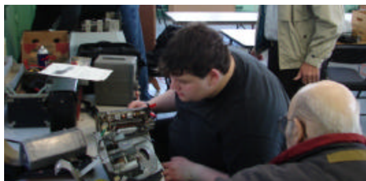
The two Johns (Tyminski and Ruccolo) work on the radio from a 1951 Desoto with 16,000 original miles. A bad vibrator was bypassed but possible IF problems still prevented a return to service.
