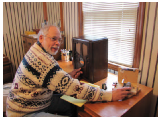
Harry Klancer adjusting a ferrite rod antenna on his Philco 38-89.
