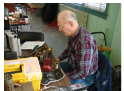
Aaron Hunter tackled a 1940 Emerson. Re-capped filters cured the hum problem but the audio failed on warm-up. The coupling capacitors are the next project.
