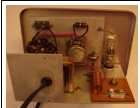
No rectification - raw ac is used for plate voltages. Notice the EM84 horizontal magic eye tube at the right.
