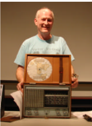
Aaron Hunter: Philco Trans-World, T-9. This is Philco's first transistorized shortwave portable radio. Dial is unique in that the logging scale slides below each band as it is selected. Troubleshooting was a problem since schematic biasing was incorrect. Radio sold for $229 in 1958 ($1690 in today's dollars).
