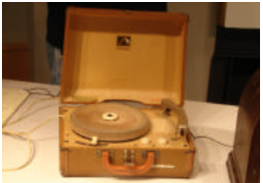
Matt Reynolds discusses this RCA portable record player with an interesting design flaw; when 33-1/3 records are played, the control knobs are covered.
