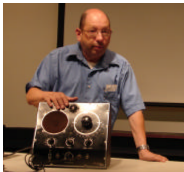
Ray Chase obtained this homebrew transconductance tube tester from a recent Estes auction; construction is first class (notice the digital displays). Its builder (D. K. Owens) even wrote an instruction manual that included a calibration procedure and schematic.
