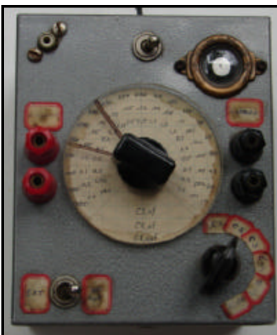
The project suggested a balance potentiometer with a scale of 0 to 100 using capacitor values read from a chart. The builder decided on a direct-reading scale.
