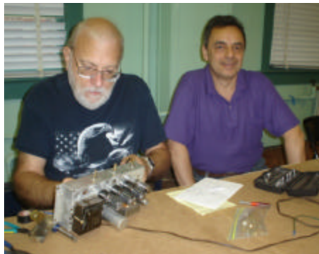
Bob Trentacoste brought in an RCA Orthophonic phonograph that required filter cap replacement and turntable servicing ... attended to by Phil Vourtsis.
