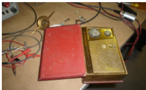
A Crosley "book" radio built with hybrid transistors and pencil tubes. The customer said it was a gift to a deceased friend from infamous mobster Sam Giancana as attested to by an inscription and initials "SMG" on inside cover.
