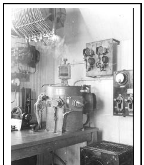
Ed was Chief Operator aboard the S.S. Etan Allen. Shown is a 2 KW Federal arc generator showing an alcohol dropper on top. The tuning coils are above and the chopper, antenna ammeter, variometer and key is on the desk.
