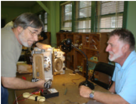
Chuck Paci and Evan Broadbelt repair a Zenith K725 AM/FM radio that just needed a tube. They were not as successful with an RCA 66X1 which was in poor state from some previous "fixes."
