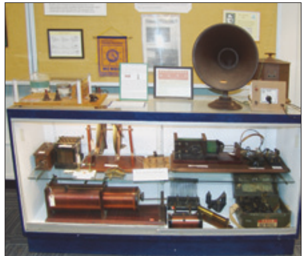
Figure 8 — An early wireless display with a working spark transmitter and crystal set receiver.
