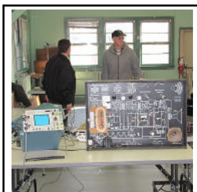
Scope station using the superheterodyne trainer.
