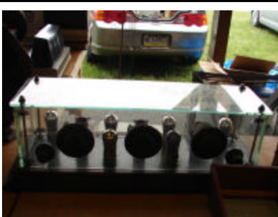
Glass radio ... some were manufactured, but many were homemade or came as kits. On this model, the wiring was not exposed.
