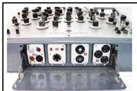
The WT-100A is supplied with four, interchangeable multiple-socket plug-in units than can accommodate up to 14 base-pin connections.
