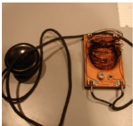
This Alva F. Allen crystal radio, entered by Dr. Mike Littman, is tuned by spreading or collapsing its coil. It originally sold for $1.50.
