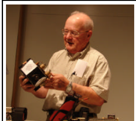
Ray Chase: This QK-390 Raytheon magnetron was used in the first commercial microwave oven. It ran at 1500 KW and 2450 MHz.
