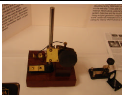
Replica Fessenden liquid barreter tested with a "Skywaves" crystal set.
