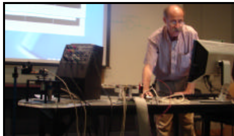
Rod held upright by feedback control.
