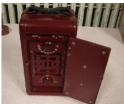
Walt Heskes talked about his 1948 Globe Model 454 "camera" AC/DC radio. For DC, it operates off 67.5V and 3V batteries.
