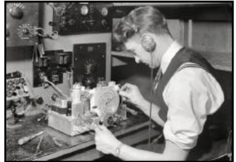
The caption reads as follows: "RCA Victor Final Inspector - testing radio frequency alignment and making final test of chassis. This takes place in a room entirely surrounded by copper screening in order to protect testing from any interference. This is the job requiring the highest skill. Even technical training, such as an electrical engineering course, must be supplemented by a course of training at the plant for this particular work."
