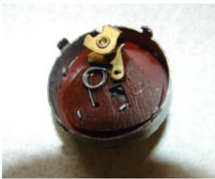
Failed switch on the Emerson DP-332. Its simple replacement avoided trying to match shaft lengths on its attached volume control.
