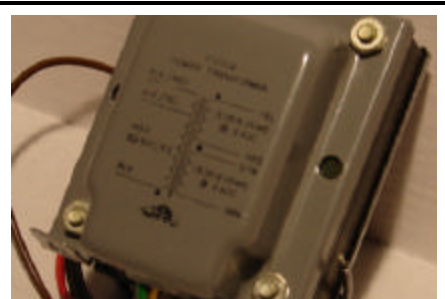
Sometimes you get lucky - a NOS low voltage power transformer with leads and values clearly marked.
