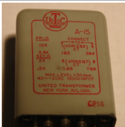
Note the "1500V HIPOT" (insulation) rating of this transformer.
