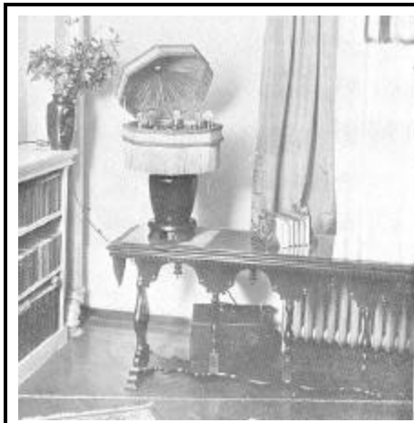
The "Radiolier" - notice what appears to be a battery box below the table and an AC line cord to the left.
