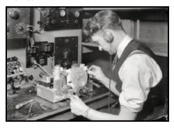
The caption reads as follows: "RCA Victor Final Inspector - testing radio frequency alignment and making final test of chassis. This takes place in a room entirely surrounded by copper screening in order to protect testing from any interference. This is the job requiring the highest skill. Even technical training, such as an electrical engineering course, must be supplemented by a course of training at the plant for this particular work."
