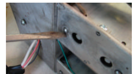
Dick Hurff's Majestic 21 nemesis...the long screw that caused a short.
