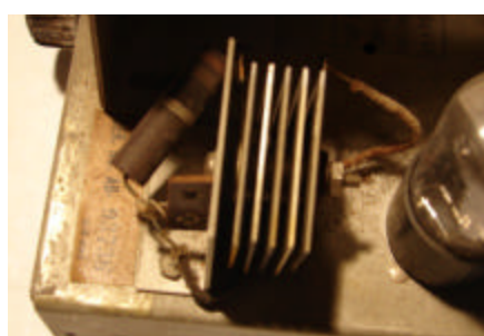
The selenium rectifier in the low voltage power supply would require replacement with solid state devices.
