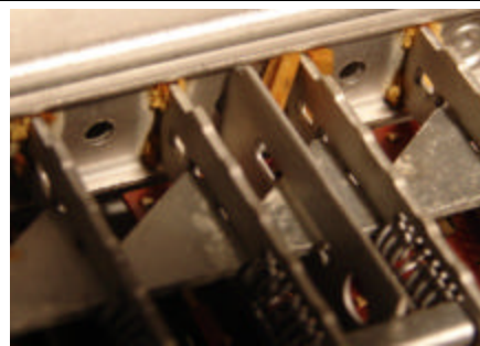
"...what appear to be brown, fiber 'necks' that surrounded each pushbutton shaft had completely deteriorated."
