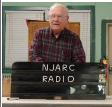
This radio frequency electronic display sign (Model 30-3C) shown by Ray Chase was manufactured by the J. Allen McDonald & Assoc. company of Pittsburg, PA. It uses two 50L6 tubes to form an oscillator that transmits a 40 kHz RF output (a "miniature tesla coil") to gas-filled character tubes that are arranged on the sign face. A box of gas filled letters from Electronic Displays of Newark, NJ comes with the sign. The original owner said that there was a short in the unit but he supplied an extra face. Ray said that he has not energized the unit and "does not intend to."
