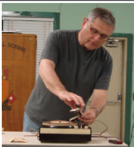
Bill Zukowski described the details of his Timex magnetic disc recorder which he bought off eBay some 10 years ago. His dad had bought one in the 50's (at $60 in 1957 dollars) but while trying to find out "where the feet grow" (a term my own dad used many times in the past), he managed to end its life. The recorder uses floppy discs, runs at 16 and 33 rpm and will even play 45's with an optional phono cartridge. The microphone was originally defective but Bill wasn't about to spend $200 for the sought after Shure control reluctance types available on eBay and installed an acceptable substitute. The discs (originally $1.49 for six) are easily erased by swiping with a common permanent magnet; "very high tech" as Bill noted.
