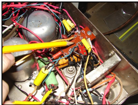
Jerry Dowgin and Al Klase attack numerous problems with an Atwater Kent 627 cathedral radio. Some poor ground connections were located and Jerry points to a fix that was constructed to solve the problem.
