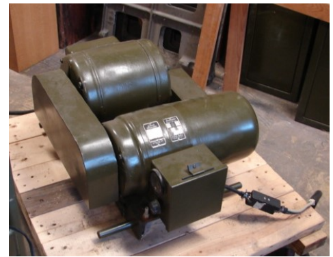
The 400 cycle power inverter.
