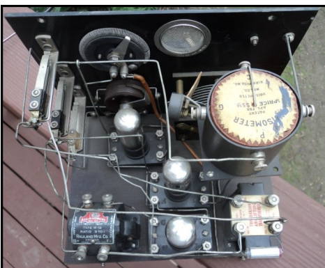
The Missouri Mystery Radio. Note the cardboard, printed voiso-meter cover as compared to the wax seal shown in the photo on page 3.
