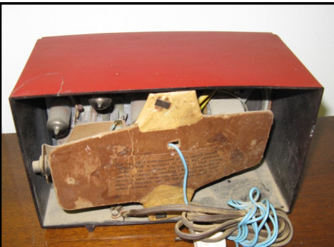
Rear view of the little red radio. Note the horizontal chassis mounting.
