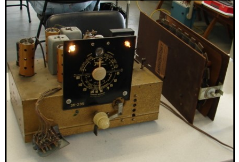
This Zenith 5808 chassis was a walk in the park for your editor. Some electrical tape and a 6X5 brought it back to working order.
