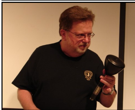
Monoscopes were special forms of video camera tubes which displayed a single still video image. They were used to generate TV test patterns and station logos. Typical was the widely used "Indian Head" test pattern. Dave Snellman displays a model 1699 which is the same as the 2F21 except for a station specific logo. The exact pattern will not be visible until the tube is energized.
