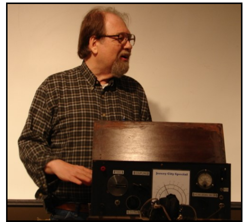
By building his "Jersey City Special" crystal set, Al Klase attempted to reproduce the early crystal-based communication receivers of some 100 years ago. Like these early sets, Al's homebrew is double-tuned with a single-tuned capability to "look around" the band. Logging some 18 stations from Jersey City, Al uses an audio transformer-coupled sound-powered headset to increase sensitivity. Al's advice: "Crystal sets are magic...build them while you can!" His presentation may be found on YouTube under "Jersey City Special."
