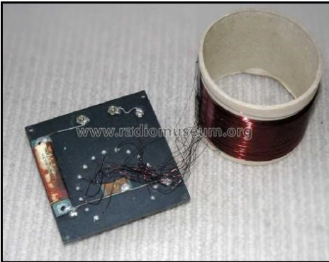
Simple internals of the Marvel crystal set courtesy of radiomuseum.org. The coil form, based on its color, may not be original.
