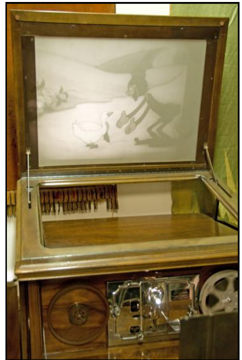
A Vitaphone "talkie" home projector using 16mm film (courtesy of Ron Hutchinson). Synchronization was accomplished by using the same drive motor for both the record player and projector.
