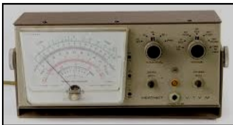
The Heathkit IM-28. It has an easily read 6" meter face and a combination AC-OHMS-DC switching test probe and ground lead that connects to a single jack. DC accuracy is +/- 3% of full scale. Unfortunately, the accuracy of the AC function of the meter is very poor for complex waveforms.
