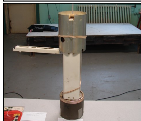
A radiosonde entered by Ray Chase. It is carried by a balloon to transmit temperature, pressure, humidity and wind speed and direction information.
