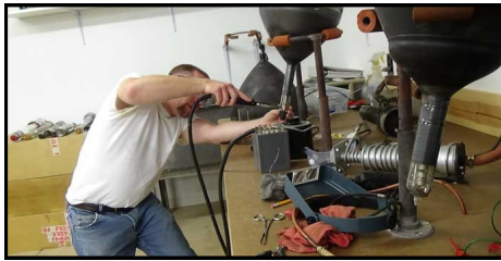
Using a wire heating device to crack the neck glass of a CRT.
