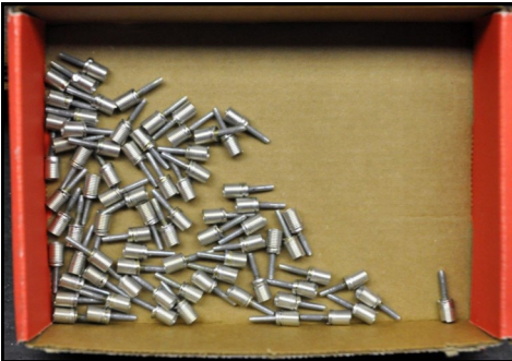
"I spent about two hours soldering springs to screws, and they came out as good as the original."
