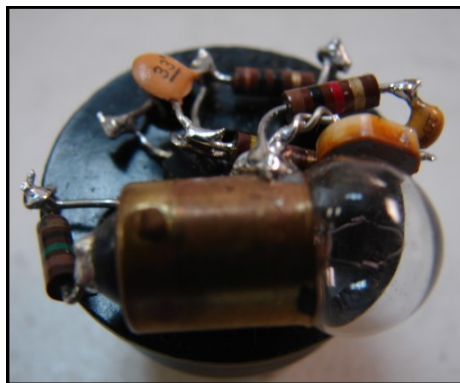
"Just for fun, I designed an experimental JFET circuit to replace the tube."
