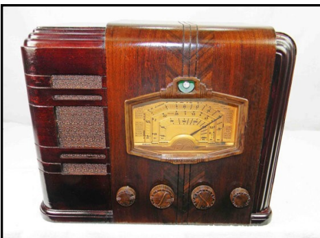
Typical six tube 1938 Silvertone 4763. It was sold as part of the "Sears Golden Jubilee" which offered a series of radios with different sized gold dials and styles. Richard described it as a TRF set but, unless I'm mistaken, it was actually a superhet with a 6A8G, 6K7G, 6B6, 6V6, 6U5 and 6X5G tube complement...Ed
