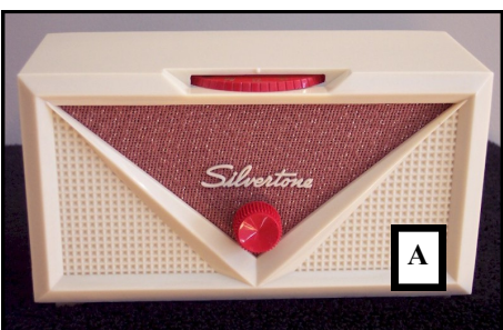
Typical six tube 1938 Silvertone 4763. It was sold as part of the "Sears Golden Jubilee" which offered a series of radios with different sized gold dials and styles. Richard described it as a TRF set but, unless I'm mistaken, it was actually a superhet with a 6A8G, 6K7G, 6B6, 6V6, 6U5 and 6X5G tube complement...Ed
