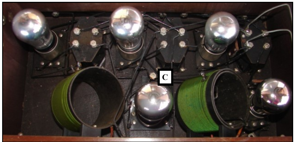
Interior of the Amrad "Neutrodyne." The single, vertical neutralizing capacitor at "C" consists of two pieces of insulated wire inside a brass tube. The tube was slid back and forth to adjust the capacitance.
