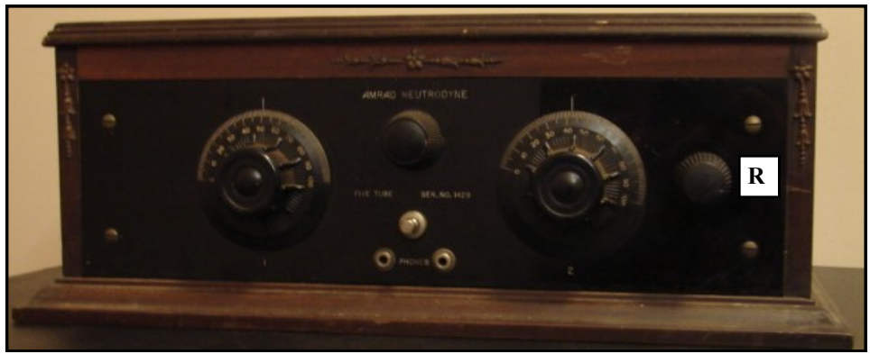
The author's Amrad "Neutrodyne." Note the "Bradleyohm-E" detector filament control at "R" which is not shown in advertised versions.
