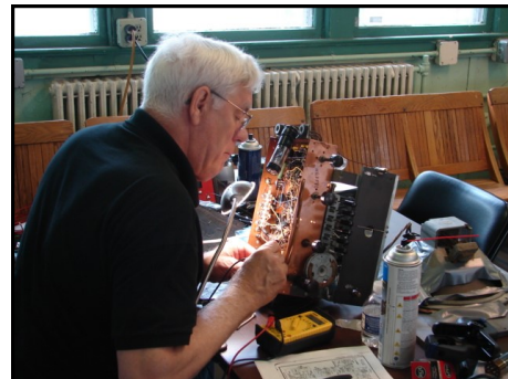
The result of mistaking a radio's antenna terminals for the AC power input. Len Newman (above) corrects an amateur's mistake.
