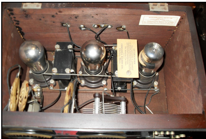
The ZR-4 "Transcontinental" with Gimbel's logo in the Mark Mittleman collection. Note that, with the exception of the slant front panel cabinet and antenna/ground connections, it duplicates the Chelsea Model 122 (RadioMuseum photo). The interior component arrangement is also exactly the same.
