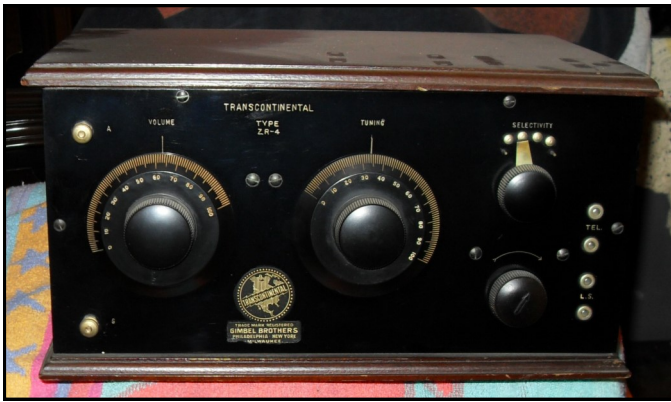
The ZR-4 "Transcontinental" with Gimbel's logo in the Mark Mittleman collection. Note that, with the exception of the slant front panel cabinet and antenna/ground connections, it duplicates the Chelsea Model 122 (RadioMuseum photo). The interior component arrangement is also exactly the same.
