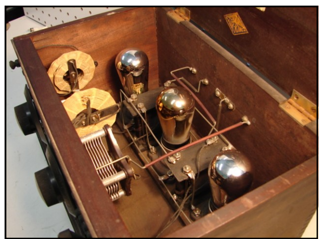
The ZR-4 "Transcontinental" with Gimbel's logo in the Mark Mittleman collection. Note that, with the exception of the slant front panel cabinet and antenna/ground connections, it duplicates the Chelsea Model 122 (RadioMuseum photo). The interior component arrangement is also exactly the same.
