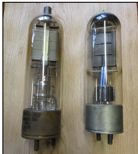
Western Electric transmitting tubes, a 219D power rectifier and a 241B triode transmitter.
