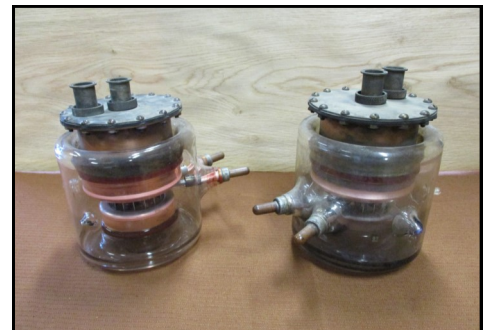
SCR-270 transmitting tubes used in the Army's first long range search radar and the one that was in operation at Pearl Harbor on December 7 th , 1941.
