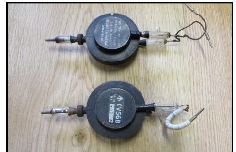
Canadian and New Zealand magnetrons used for airborne intercept and Naval search radar applications early in WWII.
