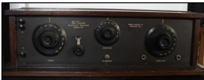
The author's Ed Nunn Model N-3. The large dial to the far right adjusts the filament voltage and is called a "Stabilizer."
