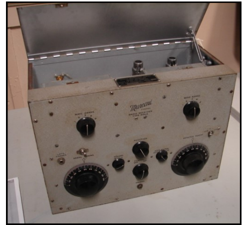
A Marconi (Canada) radio receiver, Type MSL5, 15-1500 KHz.
