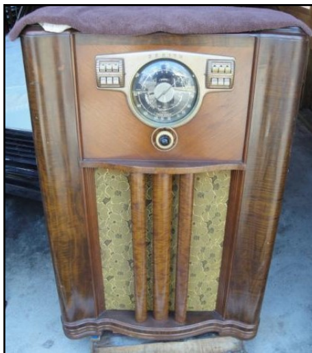
Zenith 10S569, 1941, 10-tubes, 6V6's push/pull, working.
