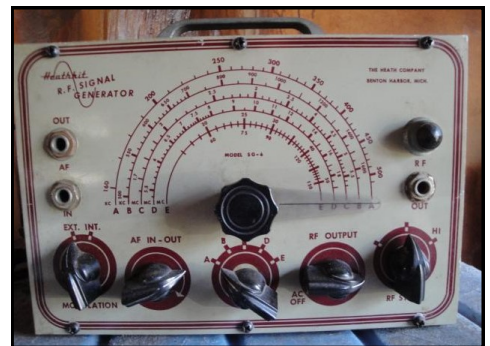
Heathkit SG-6 signal generator; untested.
