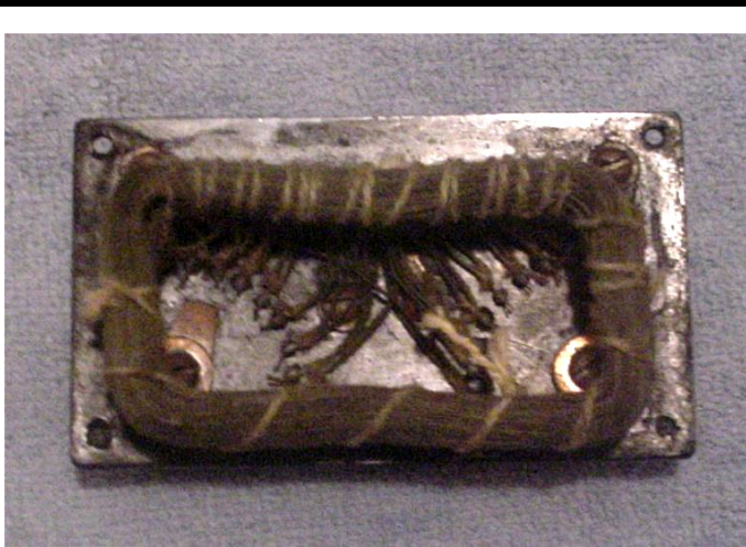
Interior of the 1924 Baby Grand showing its multi-tapped coil. With no antenna tuning, this set was designed to receive only a limited number of nearby stations. The set was available in a handsome gift box, with headphones, for $6. The set by itself, without headphones, sold for $3.40.
