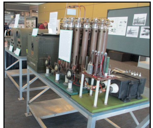
SCR-268 sixteen-tube "ring oscillator" transmitter.
